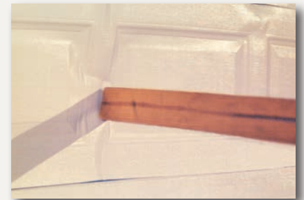
Large Missile Impact Testing
